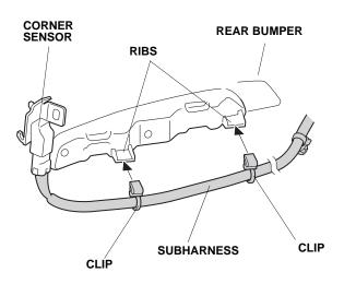
58. Secure the two clips on the subharness to the center sensor clips.
