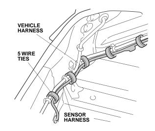
37. Install the holder to the sensor harness 6-pin connector.
