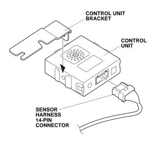
16. Plug the sensor harness 14-pin connector into the control unit.
