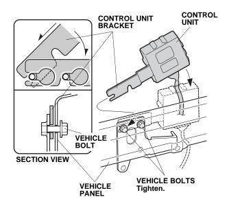
19. Tighten the two vehicle bolts.
