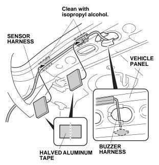
29. Cut one aluminum tape in half. Secure the sensor harness and buzzer harness to the vehicle panel using the two halves of the aluminum tape.
