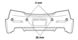
52. Remove any burrs from the drilled holes. NOTE: The sensors will not seat properly unless the burrs are removed. 53. Install two center sensors (blue) and two corner sensors (white) into the rear bumper.
