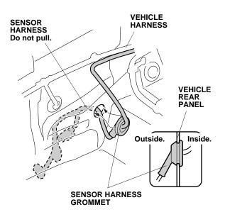
35. Route the sensor harness through the vehicle grommet hole, and seat the sensor harness grommet in the vehicle rear panel as shown. NOTE: Do not pull on the sensor harness when installing the grommet.
