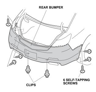
11. On each side, release the 12 hooks by gently pulling the rear bumper away from the body.
