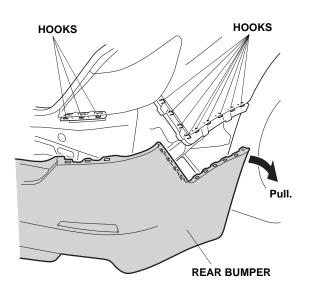
12. With the help of an assistant, remove the rear bumper (four hooks, and unplug the two vehicle connectors). Place the rear bumper on a blanket to prevent damage.
