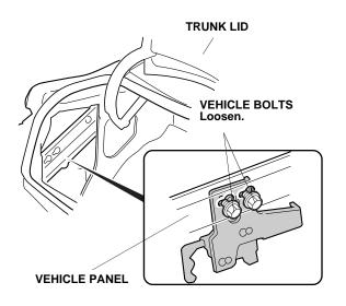
18. Slide the control unit bracket over the two vehicle bolts.
