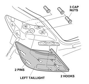
41. Release the two hooks and two pins, and pull the left taillight out toward you.
