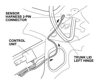
27. Plug the sensor harness 2-pin connector into the buzzer harness 2-pin connector.
