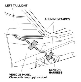
46. Secure the sensor harness to the vehicle panel using two aluminum tapes.
