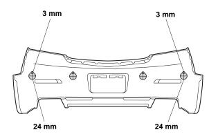
Remove any burrs from the drilled holes. NOTE: The sensors will not seat properly unless the burrs are removed.
