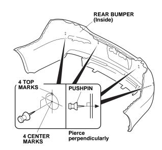
48. While wearing eye protection, use a 3 mm drill bit to drill all eight pierced points from the outside of the rear bumper.
