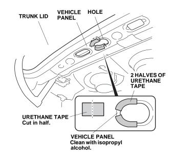
21. Cut one urethane tape in half. Attach the two halves of the urethane tape around the vehicle panel hole as shown.
