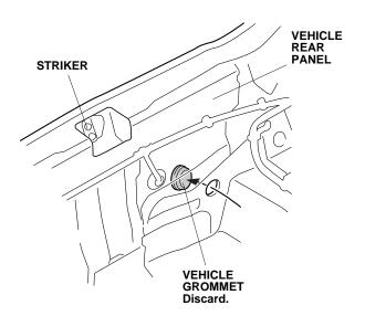
34. Route the sensor harness along the vehicle harness.
