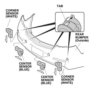
54. Install the four sensor clips.
