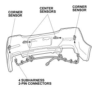
56. Secure the two clips on the subharness to the ribs on the rear bumper.
