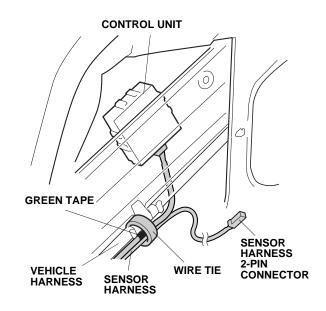
26. Route the sensor harness 2-pin connector as shown.
